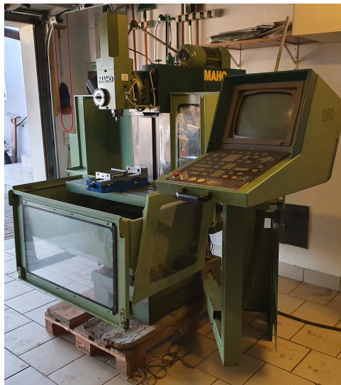
Figure 1: CNC mill Maho MH400E, built in 1984
